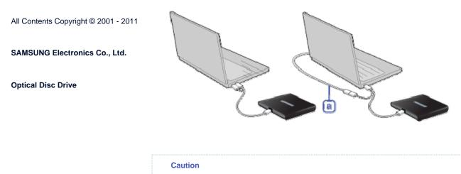
If your computer does not have a USB connector, install a USB interface card.
